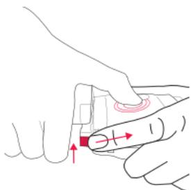
While holding both latches down, place your free hand under the recharge and your thumb on the trigger (as shown in the diagram).
