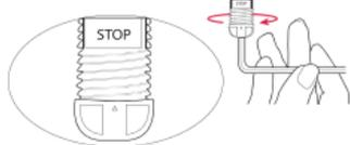
If the red marking appears, screw the cap back on a little until the red marking is no longer visible.
